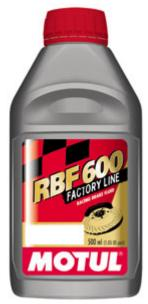
DOT 4 100% synthetic fluid for hydraulic actuated-brake and clutch systems Very high boiling point: Dry  $593^{\circ}F/312^{\circ}C$ , Wet  $420^{\circ}F/216^{\circ}C$
